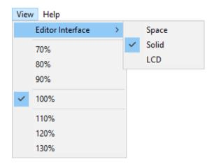
The size of the Editor Suite window can be chosen here. (The window can also be resized by left-clicking and dragging the lower-right corner.)
