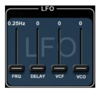
The FI4 has a dedicated Low Frequency Oscillator (LFO) for modulating the cutoff frequency of the VCF and the pitch of the VCOs. This can be used to create pitch vibrato and filter "wobbles".
