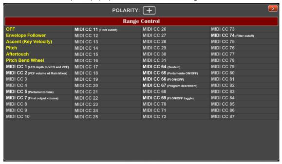
Above the list is a POLARITY button. This selects whether the range control is applied positively or negatively. By default it is positive (+). Click the button to change the polarity.
