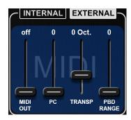
The parameters in this tab are relevant only if the FI4 is being used to convert audio signals from the input into MIDI note data in order to trigger an external MIDI synthesizer. (Please see the section on MIDI Triggering for more details.)
