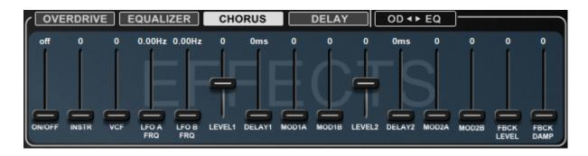
This effect is very flexible; in addition to Chorus, it can be configured as a Flanger, Slapback Echo or simple Reverb merely by setting the parameters differently.
