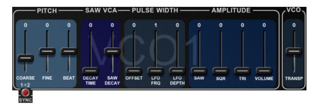
The FI4 contains four identical Voltage-Controlled Oscillators (VCOs) and these provide the basic sound source for the synthesizer. Each oscillator has three waveforms (saw, square and triangle) which can be used simultaneously. The sliders in this block adjust the tuning, volume and character of the oscillator. The oscillator blocks are located on the left-hand side of the Editor screen and, moving from left to right, their sliders are as follows:
