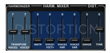
The Distortion Block applies distortion to the original instrument signal and to the three transposed voices generated by the Harmonizer.<sup>17</sup> VOICE1 is fixed at 1 octave above the input signal, whereas the transpositions of VOICE2 and VOICE3 are variable.
